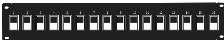
FIGURE 2-11 A Patch panel used in bulk cable installations.
